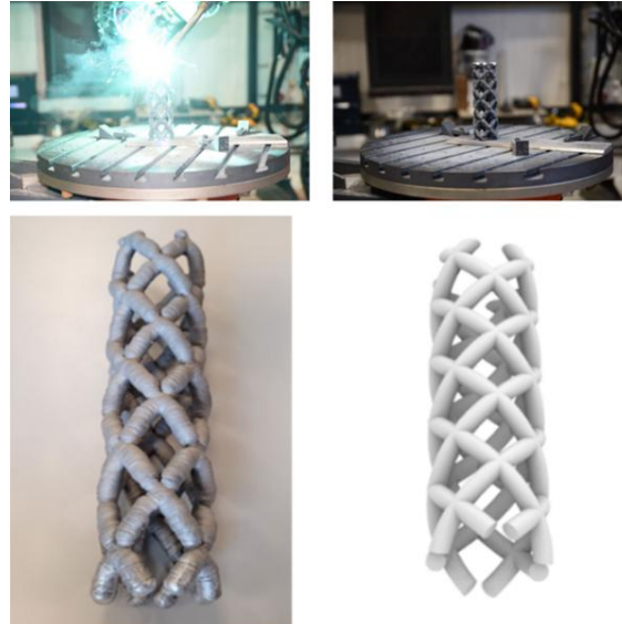
Figure 7. Image capturing the moment of spot-welding operation using PMC process. Image of the wire-arc additively manufactured load-bearing rod using the PMC process
