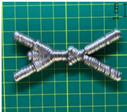
Figure 1. Visual representation of the dot-by-dot WAAM process and stickman test figure Additional pictures/information
