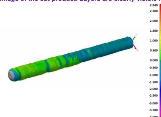
Figure 5. CMM scan geometry for a rod manufactured via WAAM. A uniform cylinder is used as a reference to compare the manufactured part, and the deviation from the uniform cylinder is shown
